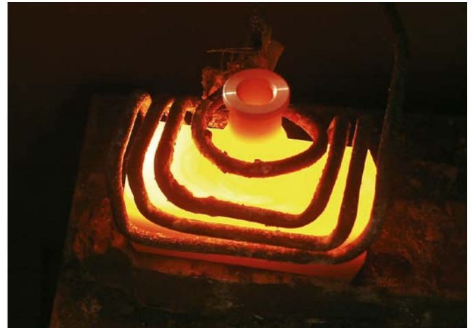
optris® CTlaser 1M/2M/3M devices used during induction-hardening
