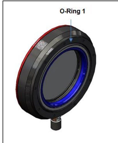
Figure 27: Insert O-ring 1 in air purge collar
